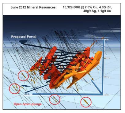
Figure 2: Stockman Cu-Zn-Ag-Au Project: Currawong Deposit - 3D isometric projection showing mineralised envelopes, drilling, planned development and down plunge mineralised intersections.
