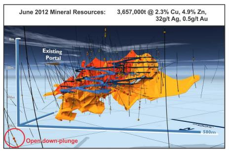
Figure 3: Stockman Cu-Zn-Ag-Au Project: Wilga Deposit - 3D isometric projection showing mineralised envelopes, drilling, planned development and down plunge mineralised intersections.
