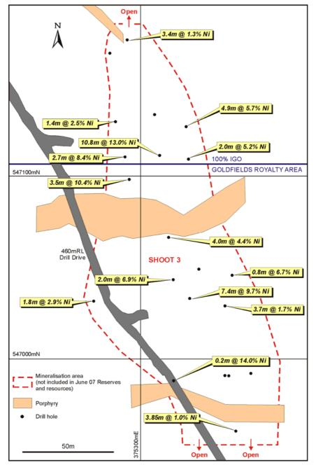
Figure 4: McLeay - Shoot 3 Plan Showing Significant Intercepts, Shoot Boundaries and Drill Drive Location. Intersection Widths are Down-hole widths
