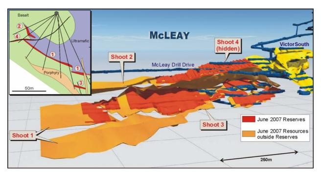
Figure 3: McLeay – 3D Isometric Model Showing Nickel Shoots
