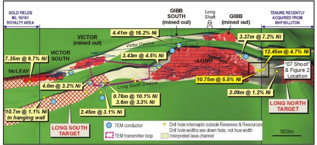
Figure 1: Long Nickel Mine – Longitudinal Section Showing New "07 Shoot" Location (Detail Figure 2), Lava Channels, and Significant Intercepts Outside Current Resources
