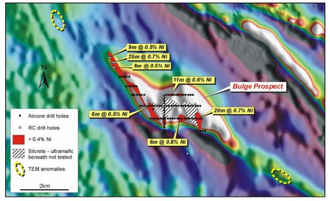
Figure 12: Duketon JV – Bulge Prospect – Drilling Results and TEM Anomalies Over Magnetic Image
