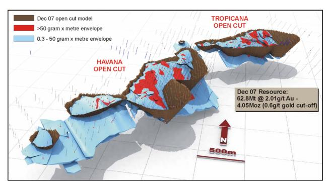
Figure 6: Tropicana JV – Isometric Model Showing 0.3g/t Au Mineralised Envelope, 50g/t Au x Thickness (m) Contours, and the December 2007 Conceptual Open-Pit Outline at a Gold Price of US\$800/oz
