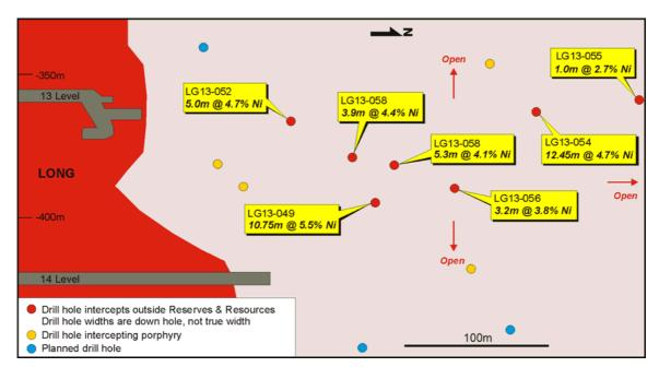
Figure 2: Long Nickel Mine – "07 Shoot" Longitudinal Section Showing Significant Intercepts, June 2007 Long Resource Boundary and Footwall Drive Locations
