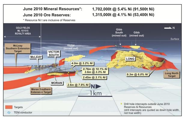
Figure 1: Long Nickel Mine – Longitudinal Projection Showing Target Areas, TEM Conductors and Significant Intercepts
