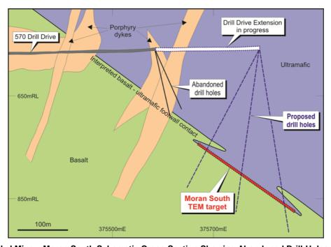
Figure 2: Long Nickel Mine – Moran South Schematic Cross-Section Showing Abandoned Drill-Holes, Proposed 570 Drill
