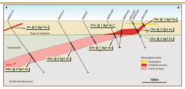
Figure 9: Karlawinda - Bibra Prospect - Cross-Section Showing Supergene, Oxidised and Primary Mineralised Zones
