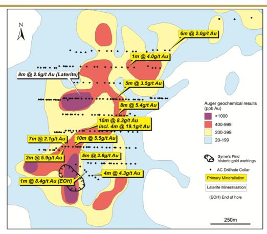
Figure 12: Holleton - Syme's Find Prospect Map Showing Significant Drill Intercepts Over Auger Geochemical Results
