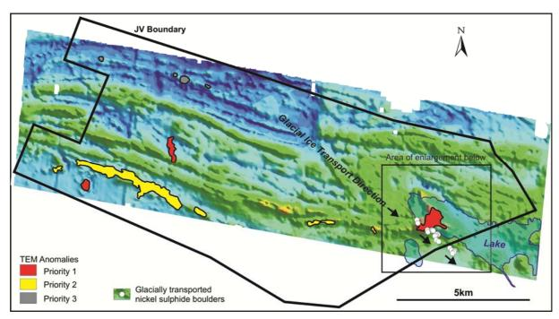
Figure 16: Orrbacken JV – 1.5km Long Nickel Sulphide Glacial Boulder Trail, JV Boundary, Lakes and Prioritised TEM Anomalies Over Aeromagnetic Image
