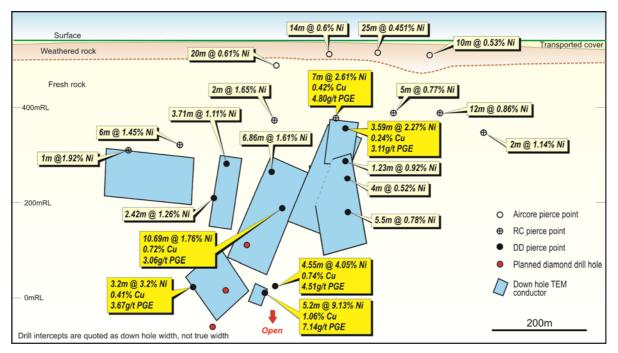
Figure 15: Duketon JV – Rosie Prospect Longitudinal Projection Showing Significant Drill Intercepts, Down-Hole TEM Conductors and Planned Phase 1 Infill Drill-Holes
